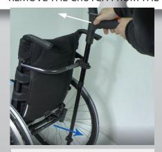
1) Push the handle of the crutch until the magnetic attachment releases from the chassis
