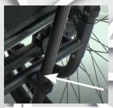
3) Move the crutch's lower attachment towards the chassis until the magnet attaches to the metal tube.
