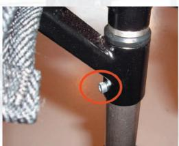
What we have done is to add two slits on the vertical tube to make it expand against the socket correctly and that the glue gets a good grip. We have also added a stop screw to strengthen the attachment even more. See lower image.
