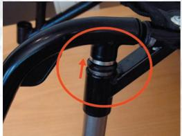
There is no risk for the attachment to come loose completely, just a small gap will occur between the vertical chassi tube's (unpainted) upper limit, and the chassi socket The function of the swing-away legrest could get less accurate.
