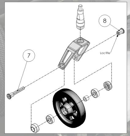
On the first 100 Panthera X delivered, an improper threadlocking (Loctite) has been used on the castor wheel bolt. (pos. 6 och 7)
