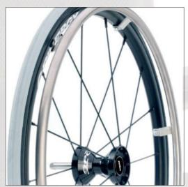
Now we replace the rear wheel axle for Spox std with the same axle we use with the new hubs on our standard rear wheel. This means that you don't need the 7 mm spacer previously used together with the old axle.
