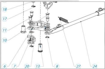
We have detected that a handful of the pull spring (no. 27) on the Panthera X brake, delivered to our customers, do not meet our requirements for quality. It might tear off after a period of use. Therefore, we would like to ask our customers to replace this spring with the new, stronger pull spring.
