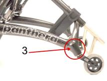
Aluminium protective sleeves should be glued to the outside of the front fork's mounting. art.no. 9024009
