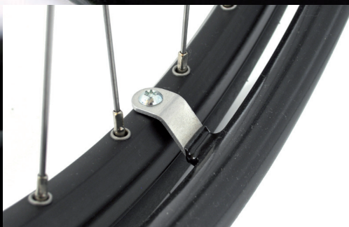
NEW PARA- AND TETRAGRIP PUSHRIMS WITH BENT TABS
