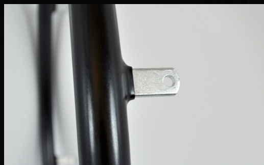
OLD PARA- AND TETRAGRIP PUSHRIMS WITH STRAIGHT TABS
