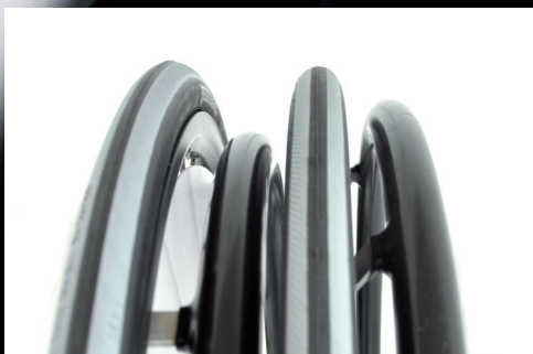
DIFFERENCE IN DIAMETER BETWEEN THE OLD PUSHRIM AND THE NEW TO THE RIGHT - 530 TO 560 MM
