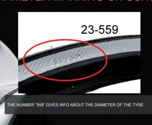
Clarifying information of how to read out the diameter on the Schwalbe tyre.
