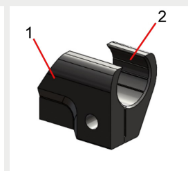
New clamp for right brake seen from outside
