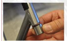
Disassemble the footrest. Cut off the desired distance of the frametube, equal on both sides. Remove all burrs.
