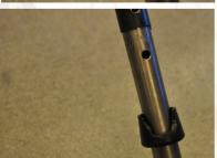
Drill new holes (dia. 5,4 mm) on the footrest on both sides, so the it can be adjusted to the desired height, NOTE! The drillholes must not be closer to each other than C-C 8 mm.
