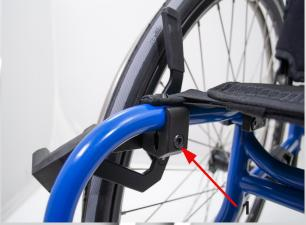
1) Mount the brake on the chassis using a 5 mm Allen key and tighten the screw (1). Do not fully tighten the screw to a start.
