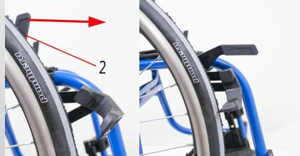
**2)** Put the brake in the activated position by moving the brake lever (**2**) forward.
