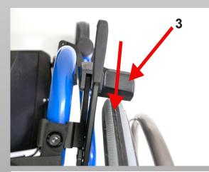
**3)** Slide the brake along the tube until the blade (**3**) touch the tire.
