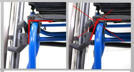
4) Check that the bracket (4) is perpendicular to the seat.
