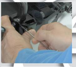
3) Fit screw M5x30 mm through the threaded bushing, welded on the chassis. Tighten with Allen key 3 mm.
