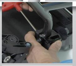
5) Tighten securely with a 4 mm Allen key.
