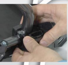
2) Put the bracket on the chassis as shown in the picture and close the bracket. See exploded view on page 3.
