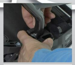
6) Take screw M5x16 mm. Put it in the other hole and tighten firmly with a 4 mm Allen key.
