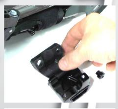
1) Remove the rear wheels and place the wheelchair upside down. Take one bracket, left or right.
