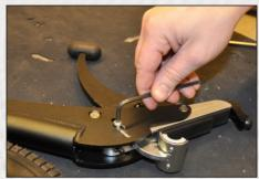
Start by loosing this screw with allen key 4 mm. Do not remove, just loosen..
