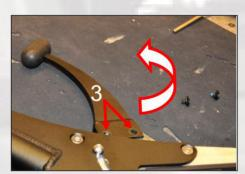
Turn the handle around 180° and reassembly the screws (3) with Loctite.
