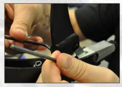
Remove the screws (3) using two allen key 4
