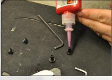
Put a drop of Loctite on the removed screws (3).
