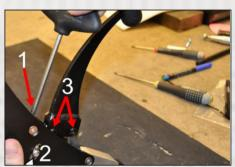
Loosen the screw (1) with allen key 5 mm, to let the screw (2) slide in the slot and in that way expose the screws (3).
