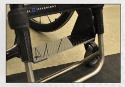
An example of an adapted footrest, where you need to turn the handle on the Freewheel around 180°
