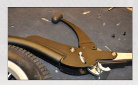
The handle on Freewheel needs , in some cases, to be turned around  $180^{\circ}$ , when it interfere with e.g. an adapted footrest to Panthera X.
