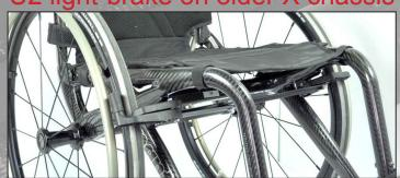
The first versions of Panthera X had a U2 light onehand brake. The assembly of this brake differs from the Panthera X brake on later Panthera X chassis.
