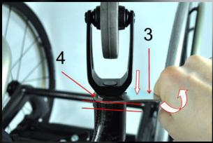
Place the special tool (3), included in the Panthera X tool box, on the "nut-lock"(4).
