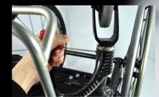
Enter the castor fork into the chassis. Align the holes (5 and 6).
