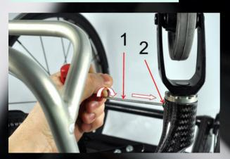
Loosen the M4 screw (2) with the Allen key 2,5 mm or the torx T20 key (1).
