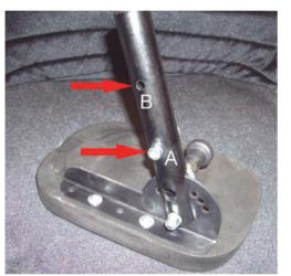
When using the amp.support on the S2 swing you need to move the stop screw "A" to position "B", to get the amp.support into the right level to the seat.
