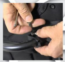
3) Fold the clamping bracket around the back rest tube and enter the counter sunk screw.
