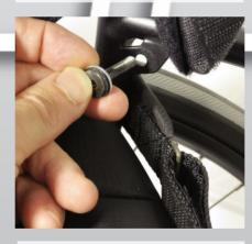
5) Mount the other screw into the hole on the ear that is welded onto the back rest tube
