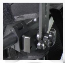
9) Mount the trunk support into the attachment.
