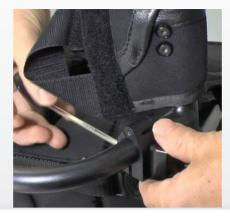
8) Tighte the screw firmly with allen key 4 mm.
