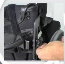
10) Adjust the trunk support to desired height abd then tighten the screws. Repeat the procedure on the other side if a left trunk support should be mounted. Finish by mounting the back rest upholstery.
