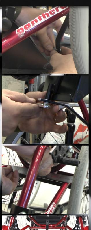
Mount screw and washer to the lower part of the stabilizer rod that should be attached to the foot plate.
