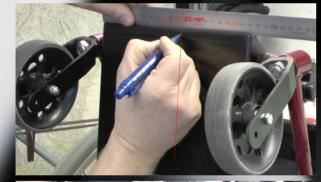
Find the center of the foot plate and add 20 mm, which is half the width of the attachment, and draw a line with a pencil.
