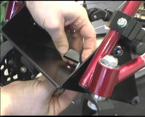
Attach the location piece with the screws. Use washers and apply a small amount of Loctite to the threads. Tighten the screws firmly.
