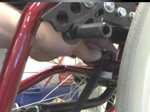
Mount the other part of the clamp and attach the satbilizer rod the the chassis as shown in the image. Mount the nyloc nut and tighten the screw slightly.
