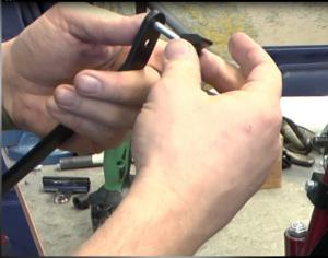
Mount the screw and one part of the clamp to the stabilizer rod that should be attached to the chassis.
