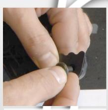
2) Mount the first screw and tighten it a few turns by hand.
