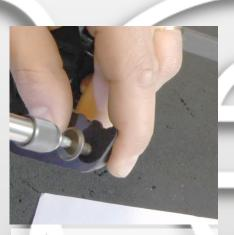
3) Tighten the screw almost to the bottom with a power tool or with a hand tool. Allen key 4 mm.
