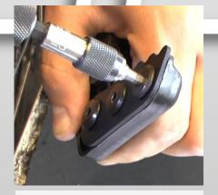
5) Finally tighten the screws firmly to the bottom.
