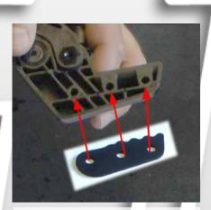
1) Place the holes of the brake blade over the holes on the underside of the S3 brake.
