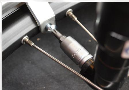
The screws must be tightened with a Torx tool (size T25). In this case an air-powered tool with a 90 degree angle head is used. NOTE! The recommended torque is 6 Nm.
