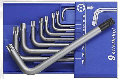
If you don't have access to an air-powered tool you can of course use a hand tool. Tighten the screw by hand until it stop then use the hand tool to tighten another quarter of a turn. It's important that the tool enters the screw entirely to avoid damage of the Torx head.
