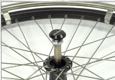
Make sure to mount the push rim on the correct side of the wheel. The push rim should be mounted on the side where the hub has a counterbore for the QR-axle.
