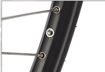
Rim with pre drilled and threaded holes. 6 in each rim.
