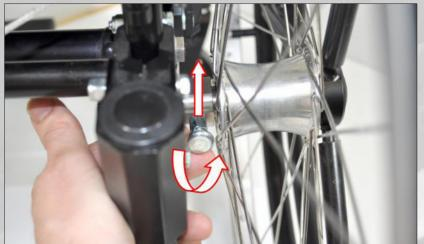
Turn the locking pin and check that it enters fully and lock the rear wheel. Check on both sides. **NOTE! Important!**
