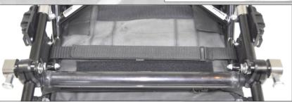
Disassemble the rear wheels and put the wheelchair up side down to access the rear axle. One arm drive with QR is mounted together with the old std rear axle, and if the chair is equipped with the Carbon rear axle, you need to replace it with the old std rear axle
