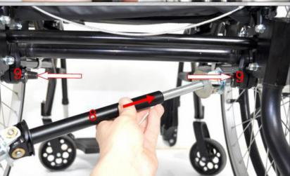
Fit the driveshaft (8) end into one of the wheel axles (9) and press the springy driveshaft to fit the other rear wheel axle. Test the function of the driveshaft by turning the smaller pushrim to see if it drives the wheel on the other side.
