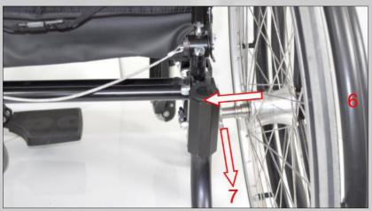
Assemble the rear wheel with push rims (6) on the side that suits the user. Enter the rear wheel axle into the attachment and at the same time pulling out the locking pin (7). Check that the axle is fully inserted. Repeat on the other wheel.
