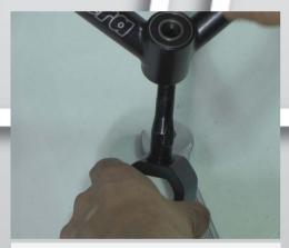
4) Mount the new castor fork into the attachment on the wheelchair.
