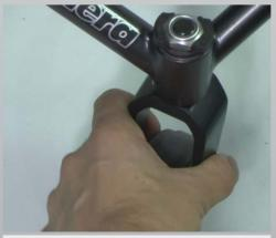
8) Check that there is no play between the fork axle and the bearing housing and that it swivels easily.
