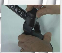
1) Remove the plastic cover from the locking nut. You might need a table knife to bend it loose.
