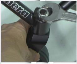
2) Unscrew the nut with a 19 mm spanner.
