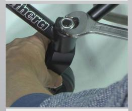
7) Tighten the nut slightly with a 19 mm spanner.
