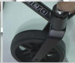
6) Put the cover plate and the nut onto the threaded castor fork axle.
