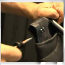
1) Use a screw driver and punsh a hole in the plastic knob in the backrest tube. and pull it out.
