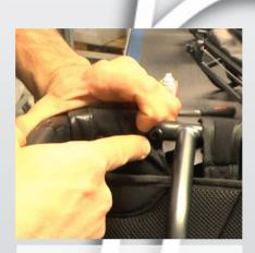
2) Place one of the push handles into the backrest tube and pull away the upholstery to free the threaded hole.
