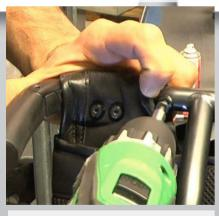
4) Finally tighten the screw firmly using the power tool with allaen key 4 mm.
