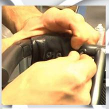
3) Mount the screw into the hole and tighten it by hand for appr. 5 turns.
