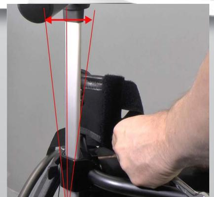
5) If the angle of the push handle needs to be adjusted, you can turn the eccentric metal cup with a 10 mm spanner.. Start with loosen the screw that holds the attachment, a bit.
