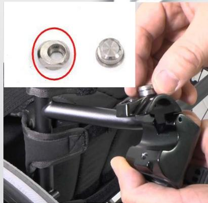
2) Bring out an attachment, there is a left and a right version, place the "open" metal cup into big hole in the attachment, from the outside.
