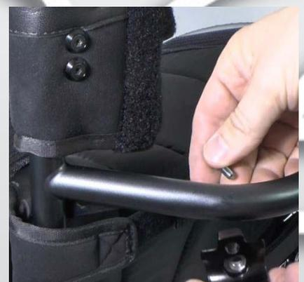
3) Open the attachment and place it around the backrest tube. Let the metal cup guide the attachment onto the knob on the backside of the tube. Mount the smaller M4 screw through the metal cup into the threaded knob
