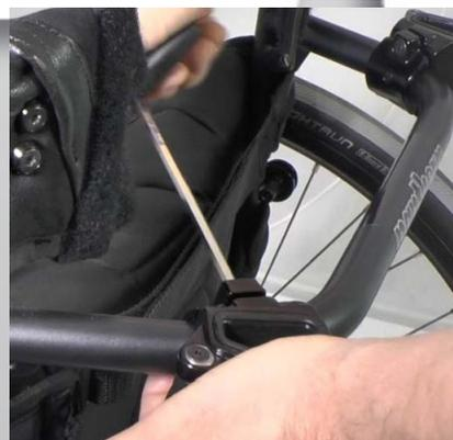
4) Tighten the screw slightly with allen key 4 mm.
