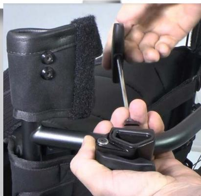
5) Then mount the larger M5 screw in the upper hole, that holds the attachment together, with allen key 4 mm. Then tighten both the M4 and M5 screws firmly. Repeat the procedure on the other side.
