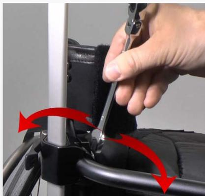
6) Use a 10 mm spanner and turn the metal cup forwards or backwards until the push handle is vertical.
