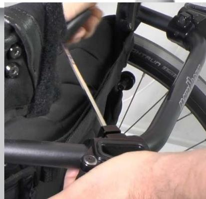
4) Tighten the screw with allen key 4 mm. Repeat the procedure on the right side.
