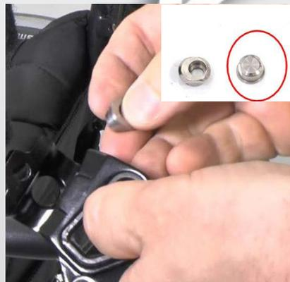
2) Bring out an attachment, there is a left and a right version, place the "closed" metal cup into big hole in the attachment, from the inside.
