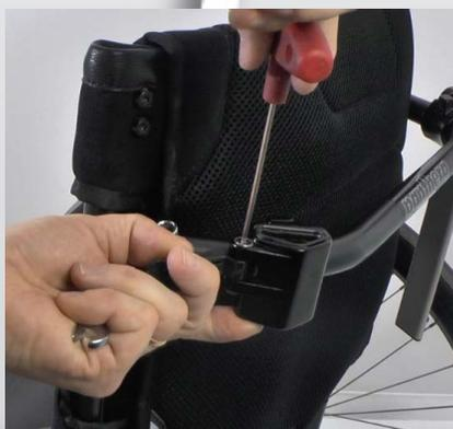
2) Disassemble the push handle. Loosen this screw a few turns with allen key 2.5 mm.
