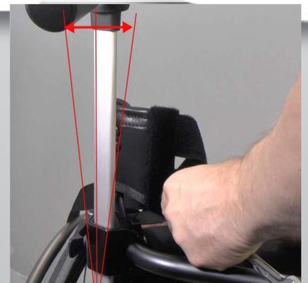
5) If the angle of the push handle needs to be adjusted, you can turn the excentric metal cup with a 10 mm spanner.. Start with loosen the screw that holds the attachment, a bit.
