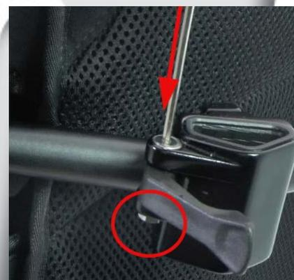
3) Push the screw downwards until the nut on the underside gets visible
