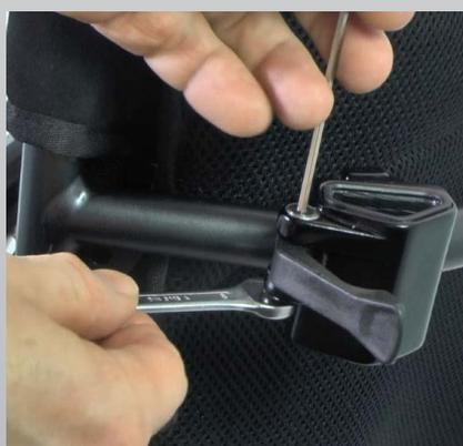
4) Adjust the locking force by turning the nut anti-clockwise (seen from the top) to increase it, and clockwise to decrease the locking force. Turn the nut a quarter of a turn, using a 8 mm spanner, tighten the screw and test it..
