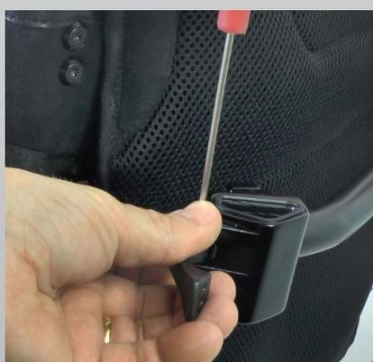
5) Tighten the screw and make sure that the nut slides into the attachment properly.
