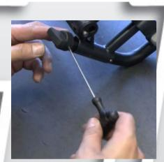
1) DISASSEMBLY Start with loosning the knob with allen key 2.5mm
