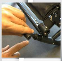
5) Bring out the special tool and use it to lift the spring loaded hose. When its extended, remove the rivet and let the hose slide down into the anti-tip. If you don't have the special tool you can use an old wheel spoke. LINK
