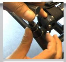
4) In the extended position place the rivet into the hole. When the hose is locket, pull out the special tool.
