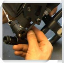
4) Tighten the screw that lock the anti-tip on the frame firmly.
