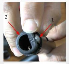
1) ASSEMBLY Bring out the new anti-tip and note that they are marked with "R" for Right and "L" for Left side.. Use the rivet (1) to lock the hose in an extended position (2).
