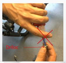
3) The locking screw for the anti-tip is treated with Dri-Loc, and need therefor no extra Loctite before mounting.
