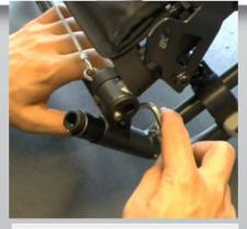
5) Loose and remove the locking screw for the anti-tip.
