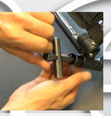
3) Bring out the special tool and put it into the anti-tip tube and by turning the knob catch the spring loaded hose and lift it up. If you don't have the special tool you can use an old wheel spoke. LINK
