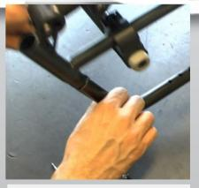
6) Pull out the anti-tip from the frame.
