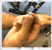
2) Bring out the locking rivet included with the new anti-tip. It should be used to lock the spring loaded inside the an-tip in an extended position.
