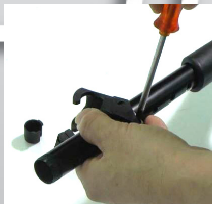
4) Tighten one of the screws slightly. With a small philips head screw driver. (Bits PH 0) or Torx TT10
