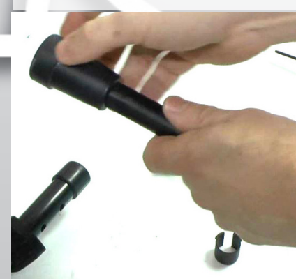
6) Remove the rubber shoe from the lower part of the crutch.
