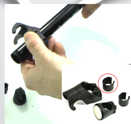
3) Slide the upper attachment onto the upper part of the crutch. The upper attachment fits tube diameter 19 to 22 mm, including the plastic bushings.
