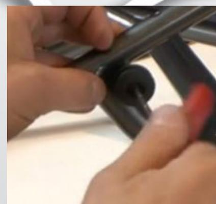
3) Tighten the screw with allen key 3 mm.
