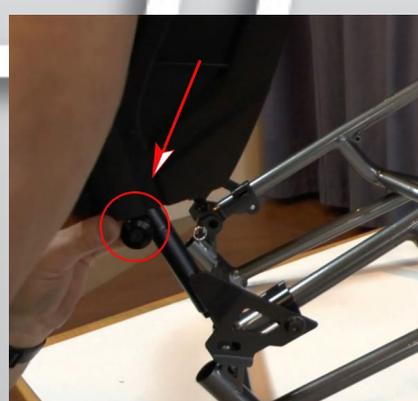
5) Bring out the right side guard and slide the slot onto the rear attachment.
