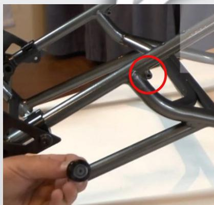
2) Start to mount the front attachment, in the threaded hole located in the front of the frame on the right side.
