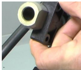
CHAMFER ON REAR AXLE AGAINST CHAMFER ON PART 4
