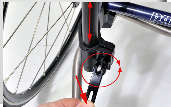
Fig. 8 Adjust it to desired height and lock it by pushing the lever down. If the lever is too loose or too tight you can adjust the pre-tension by turning it clock wise or anti clockwise. Turn it clock wise to increase the pre-tension.
