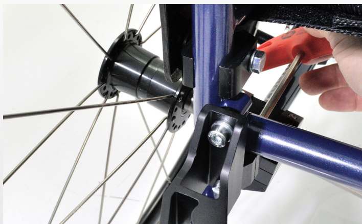
Fig. 5 Tighten the front screw that holds the attachment around the tube with allen key 5 mm.
