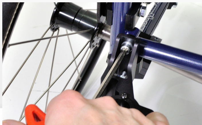
Fig. 6 Tighten the rear screw that holds the attachment to the th-readed hose with allen key 5 mm
